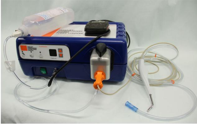
Fig 1: The hydrosurgical system (Versajet™)<sup>a</sup> consists of a foot-pedal-activated power console, a handpiece connected to sterile saline and a waste tube.
