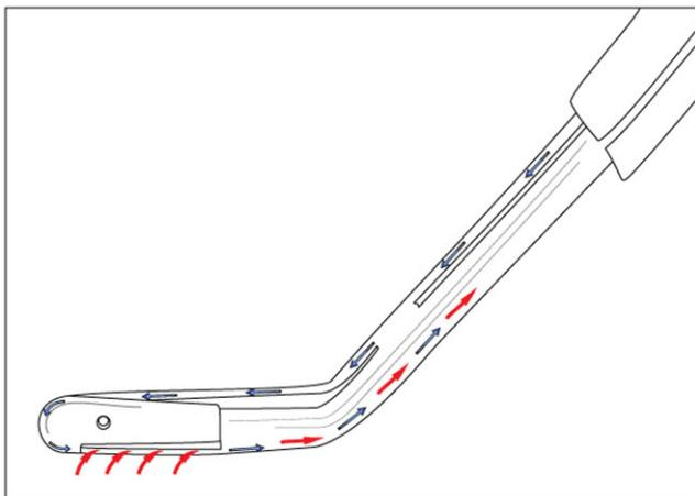
Fig 2: The tip of a hydrosurgical handpiece (Versajet™)<sup>a</sup>. A high-pressure stream of sterile saline jets across the operating window of the handpiece, creating a localised suction effect. (Illustrated by Susanne Lindeborg.)
